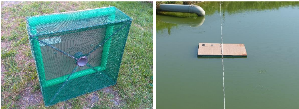
FIGURE 3. Trap created and tested to improve the catch rate of African clawed frog tadpoles
